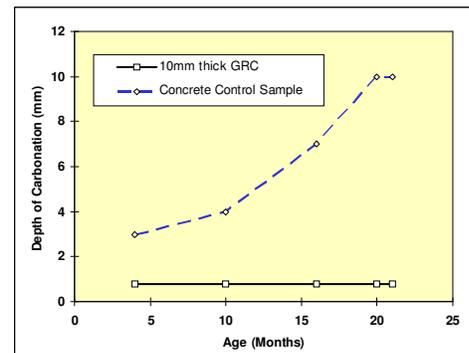
Comparative Depth of Carbonation in Accelerated Testing
