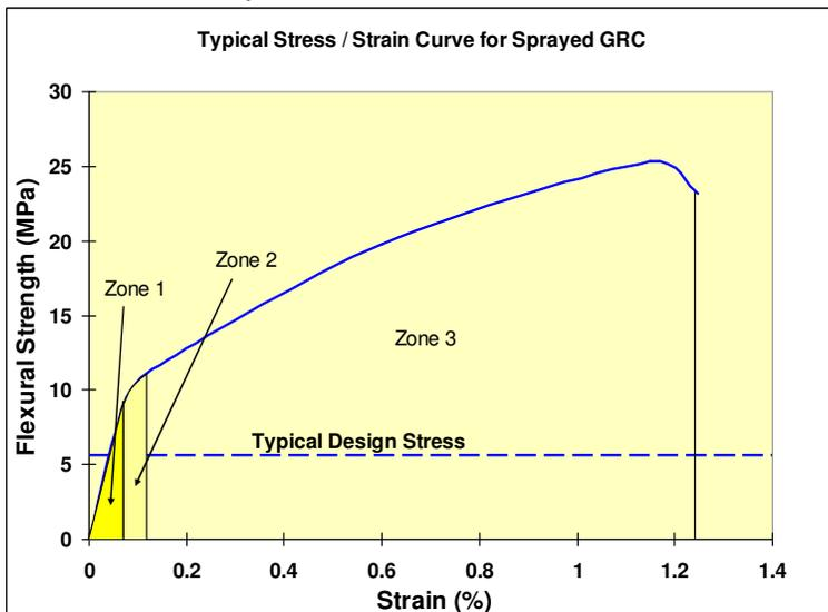
Fig. 1 Typical Flexural Stress / Strain Curve at 28 days
